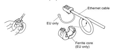
2) Pass the fastener through the ferrite core.
