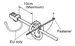
3 Loop the fastener around the cable and lock it. Use scissors to cut off any excess.
